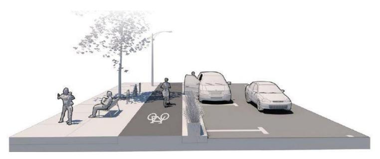
Figure 23. Illustration of a Sidewalk Level Protected Bike Lane for Third Avenue. Source: BC Active Transportation Design Guide, 2019.
