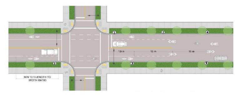
Figure 10. Painted bicycle lane to bicycle boulevard transition for Toronto Street / Highway 16, Source: BC Active Transportation Design Guide, 2019.
