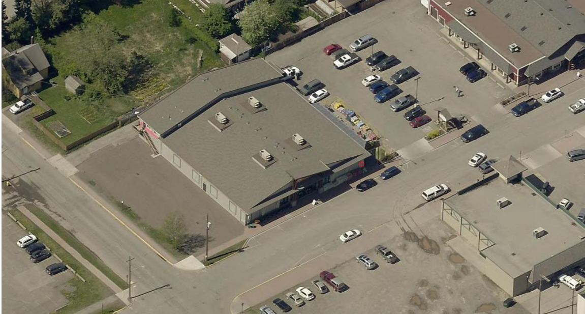
Image.4 Aerial view of the Home Hardware parking arrangement on Third Avenue; the development created on-street parking stalls by widening the abutting portion of Third Avenue in 2018.
